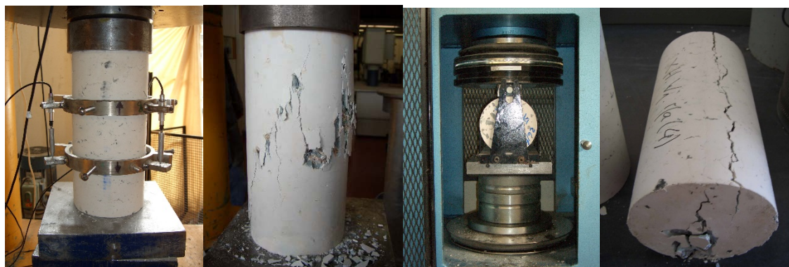
Figure 6 – Compressive and tensile tests and respectively rupture failure
