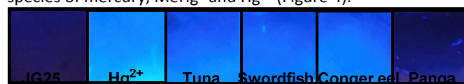
Figure 4. From left to right, polymer samples of JG25 in contact with: water ( JG25 ), a solution of \text{Hg}(\text{ClO}_4)_2 , 2.5 \times 10^{-3} M ( \text{Hg}^{2+} ), fish samples (Tuna), (Swordfish), (Conger eel), (Panga) for 20 minutes in contact with every fish sample or \text{Hg}^{2+} solution; all samples under UV light, \lambda_{\text{exc}} = 366 nm.
