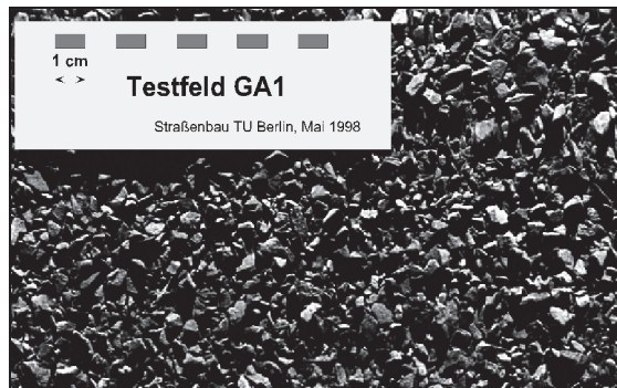
Figure 4.3: GA1 – Mastic asphalt (Gussasphalt) 0/11 with graywacke 2/5.
