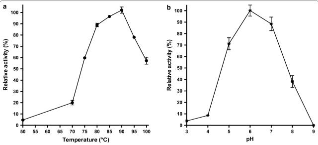
**Fig. 3** a Determination of the TtGalA catalytic activity in the temperature range of 50 to 100 °C. pNP-α-D-galactopyranoside was used as substrate dissolved in 50 mM sodium phosphate buffer pH 6.0. Relative activity at 90 °C was considered as 100%. **b** The relative activity was measured between pH 3.0 and pH 9.0, at 90 °C considering as 100% the activity at pH 6.0
