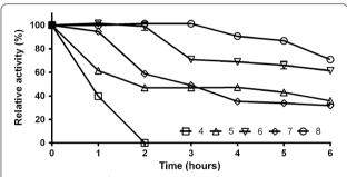
**Fig. 4** pH stability of *Tt*GalA. The enzyme was incubated in various buffers (pH 4–8) and aliquots of different time intervals were used for the residual activity assay
