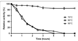
**Fig. 5** Thermal inactivation of TtGalA. The purified enzyme from T. thermophilus was incubated in 20 mM sodium-phosphate buffer pH 6.0 at 90, 80 and 70 °C for different period of time and then assayed for residual activity at 90 °C
