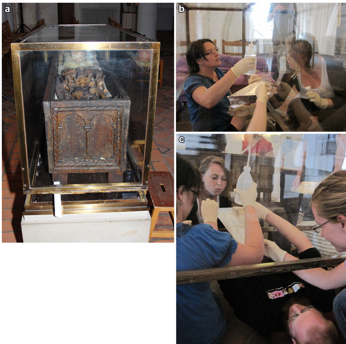
Fig. 1 a The nineteenth century show case holding the remains of King Canute the Holy (died AD 1186) in Odense Cathedral, Denmark. The folding and groove of the 100 kg heavy brass and glass show case can be seen at the lower center (Photo: Kaare Lund Rasmussen). b Applying the flush water on the interior glass wall of the show case—side view (Photo: Kaare Lund Rasmussen). c Applying the flush water on the interior glass wall of the show case—view from the back (Photo: Kaare Lund Rasmussen)
