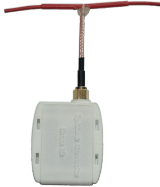
Figure 7: The DroneID device developed in the fall 2015. The external GPS antenna is described in section 4.3.3.
