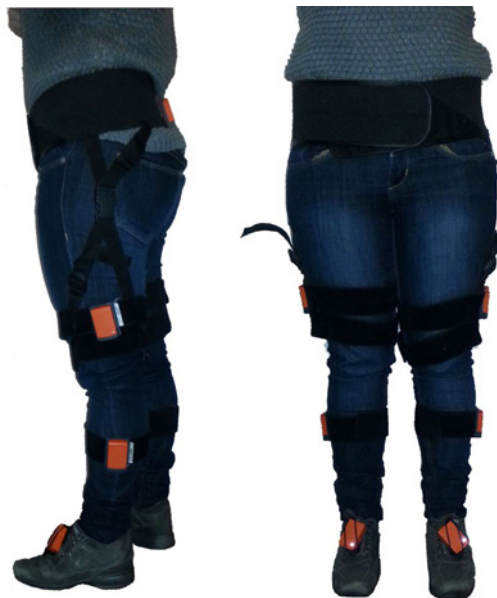
Fig 1. Position of each MIMU on one subject.
