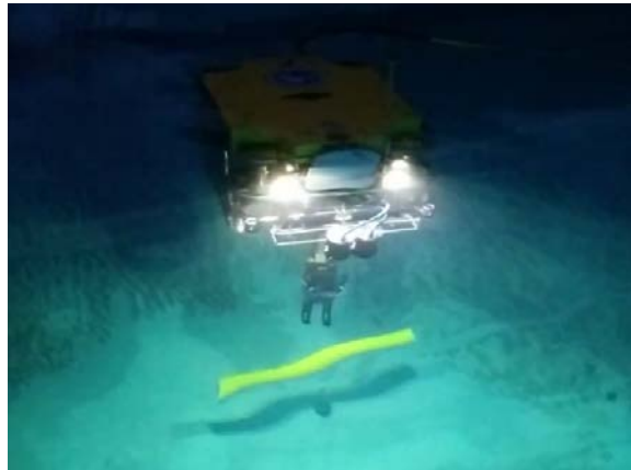
Fig. 4: Underwater view of single-agent experimental grasp operation
