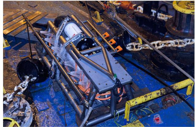
**Fig. 3** An image of Cable Termination Frame on the ship deck prior to its deployment
