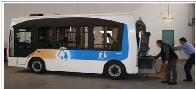
Fig. 5. Battery replacement at midday stop for the Gulliver minibus.
