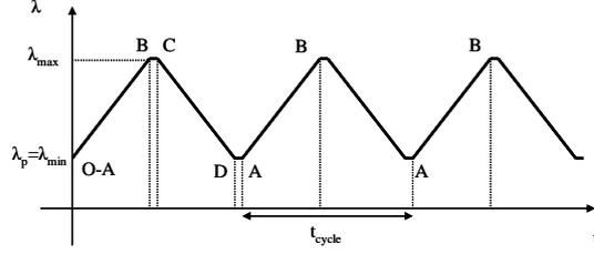
Fig. 20. Recommended time (t)-stretch ( $\lambda$ ) curve for a DEG. The maximum and minimum stretches are respectively reached at states B and A defined in the previous figure. The duration of the electrical charging (BC) and discharging (DA) phases must be shorter than the mechanical period  $t_{cycle}$ , so as to reduce the influence of electric losses through the dielectric. A constant strain rate  $\dot{\lambda}$  should be adopted during the stretching (AB) and relaxation (CD) phases.
