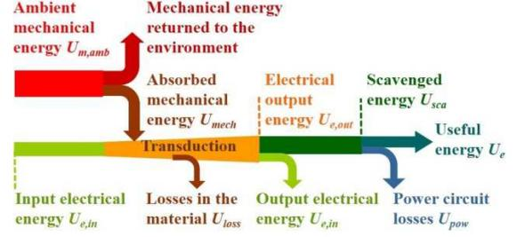
Fig. 21. Energy conversion chain and losses for a DEG.
