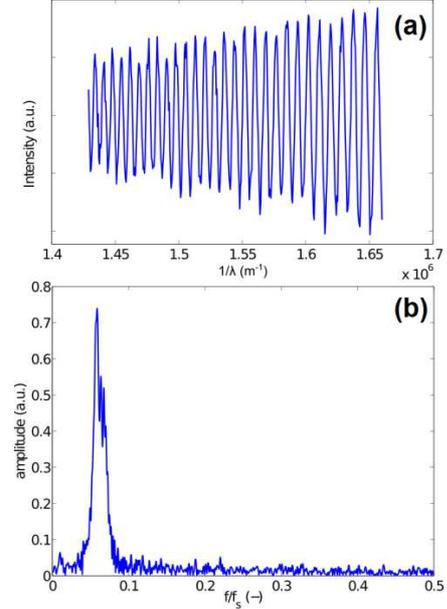
Fig. 2. (a) Transmission of a light beam through a thin PDMS: intensity is plotted as a function of  $1/\lambda$ . (b) A fast Fourier transform algorithm returns the spectrum of the signal (sampling frequency  $f_s = 2\text{mm}$ ), which shows a peak at the frequency  $0.059f_s = 0.118\text{mm}$ . Assuming a refractive index  $n=1.43$ , this leads to a film thickness  $d=41.3\mu\text{m}$ .
