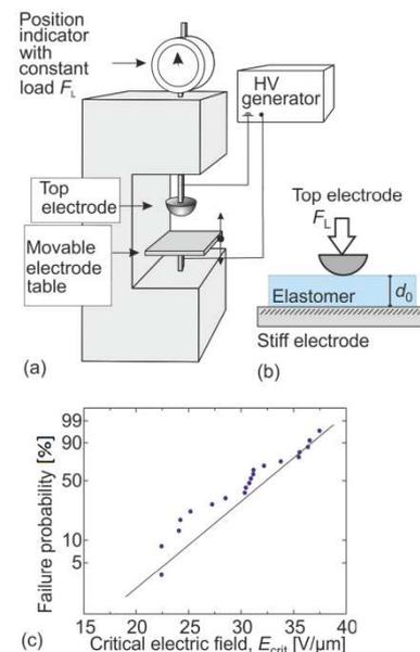
Fig. 4. (a) Schematic drawing of an apparatus to measure the breakdown strength of elastomers. (b) Hemispherical top electrode which rests with known force  $F_L$  on the elastomer film of initial thickness  $d_0$ . (c) Example of data analysis using a Weibull plot.
