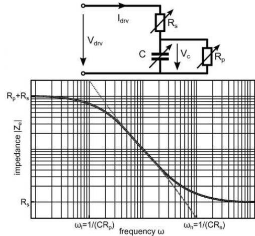
Fig. 15. Simplified electrical equivalent circuit and plot of the corresponding electrical impedance versus frequency.
