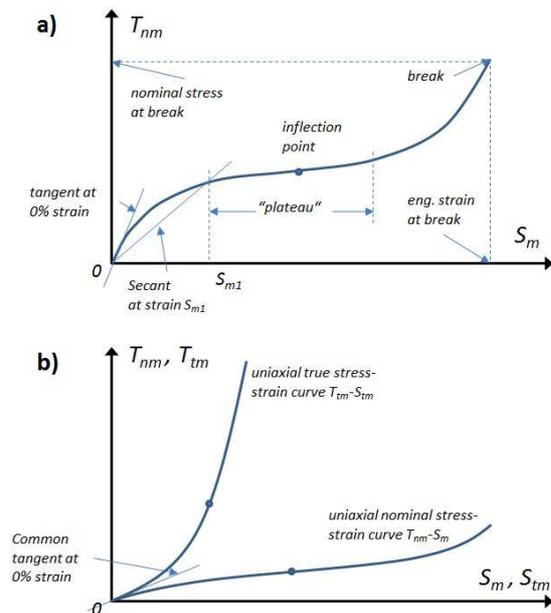
Fig. 5. a) Sketch of a typical uniaxial tensile nominal stress  $T_{nm}$  versus nominal strain  $S_m$  curve of a cross-linked elastomer. The Young's modulus  $Y$  corresponds to the tangent at 0% strain. b) Comparison between uniaxial nominal stress  $T_{nm}$  and true stress  $T_{tm}$  versus strain curves; the inclination of the tangent at the origin coincides for the two plots.
