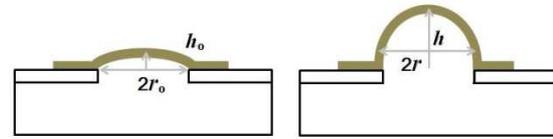
Fig. 11. Diaphragm DEA in the non-activated state (left) and in an electrically activated state (right). The internal pneumatic pressure is kept constant and small.
