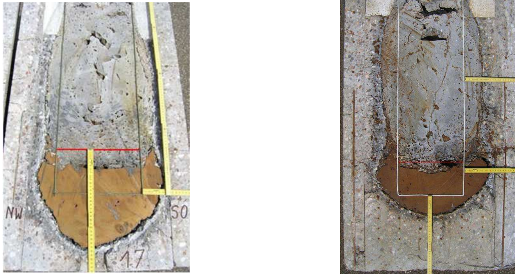
Figure 4: MOCKA Experiments showing post-test cut views with initial cavity positions (left: test without rebar; right: test with rebar)
