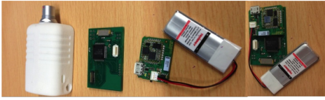
Fig. 3. From left to right: goniometer box, goniometer board, Wireless IMU + battery, IMU attached to goniometer board.
