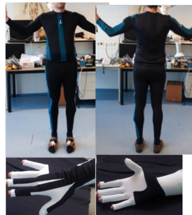
Fig. 2. Modular and wireless INTERACTION textile-integrated sensing system. Upper figures: shirt, trousers and shoes. Lower figures: kinaesthetic and kinetic glove
