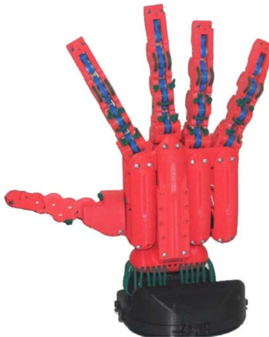
Fig. 1. Skeleton of the Pisa/IIT SoftHand advanced anthropomorphic hand prototype implementing one adaptive synergy. The prototype dimensions are comparable to those of the hand of an adult human.
