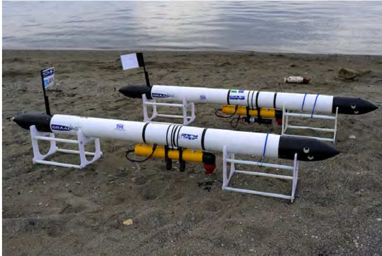
Figure 4: Folagas on shore; the UAN module is visible, mounted at mid-vehicle.
