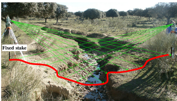
Fig. 3. An example of a measured cross-section with the use of a laser total station. The continuous line indicates the cross-section perimeter and the dotted lines indicate the point of view of the total station.
