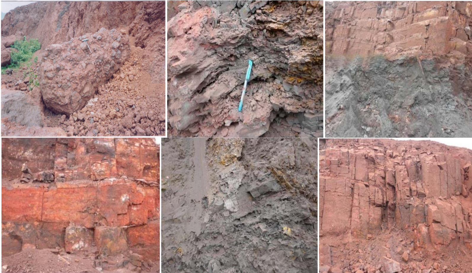
Fig. 2.4: Field Photographs showing (a) Canga ore as top cappings (b) Biscuity ore along joint pattern (c) Litho contact between hard massive ore & Blue dust (d) Hard massive ore (e) Soft Laminated Ore retaining the banding (f) Highly jointed (2 sets) hard massive ore.
