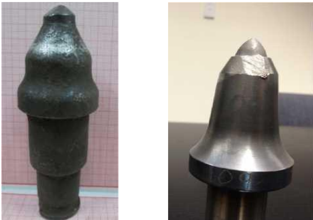
Figure 3. Early wear of a pick body around the tip
