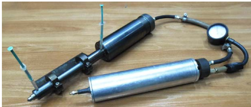
Figure 6. Pneumatic burnishing tool with a receiver (bellows with compressed air is an actuator).
