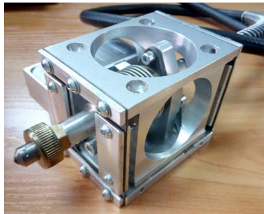
Figure 8. Pneumatic burnishing tool with a receiver (actuator is a bellows with compressed air) and a parallelogram-type mounting of the indenter on four flat posts.
