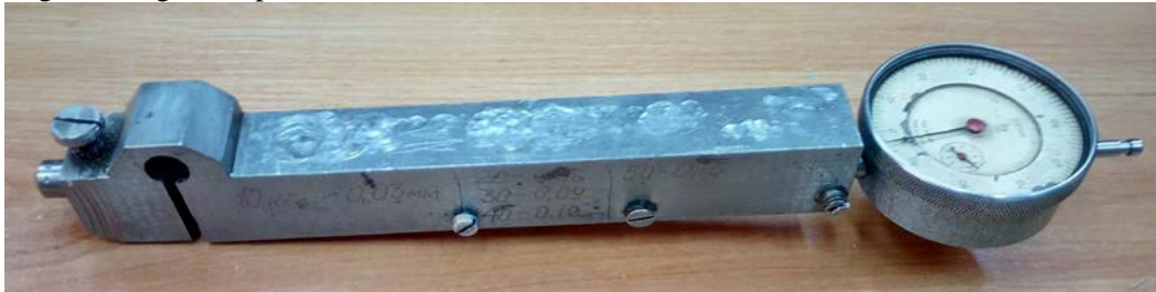
Figure 1. Dynamometric burnishing tool (an actuator is a flat spring with a vibration damper).
