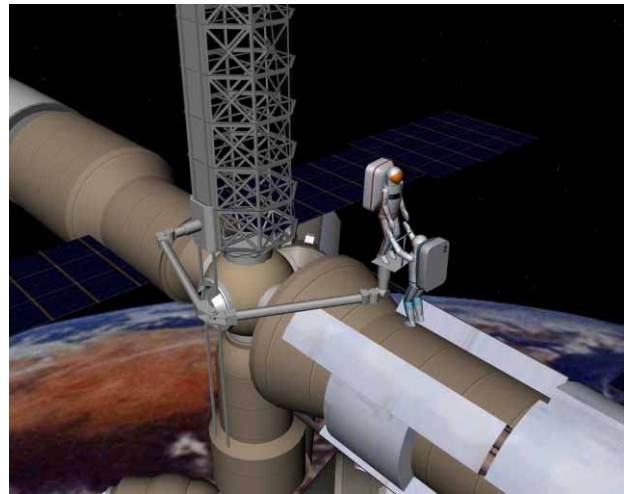
Figure 1: ERA on the Russian Segment of International Space Station, operated with two cosmonauts in EVA
