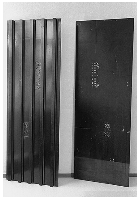
Figure 7: Skin repair and skin-doubler repair in I-stiffened panel
