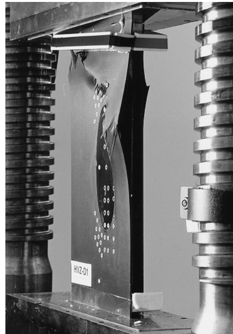
Figure 5: Failed intermediately loaded panel repair (specimen I-stiff-1)
