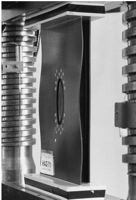
Figure 4: I-stiffened panel with a skin repair subject to 120% DUL (692 kN) in compression (specimen I-skin-2)
