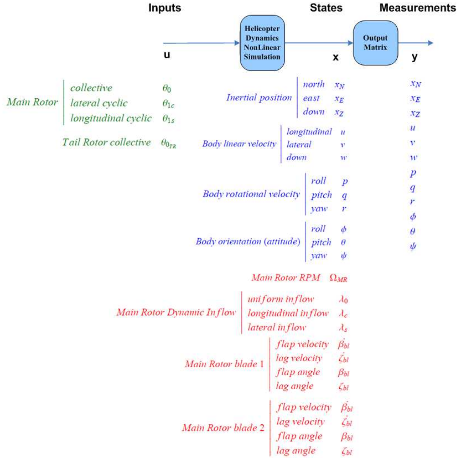
Figure 2: Helicopter Inputs \mathbf{u} (in green), States \mathbf{x} (in blue the rigid-body states, in red the main rotor states), and Measurements \mathbf{y} (measured states)
