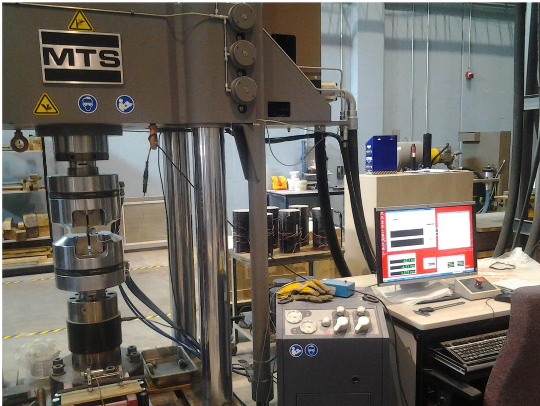
Figure D.1 Essai de traction
