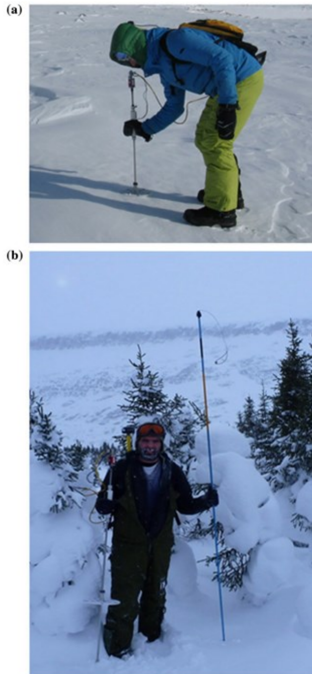
Figure 4. Measuring snow depth in the tundra snow (left) and forested area (right) using the magnaprobe.
