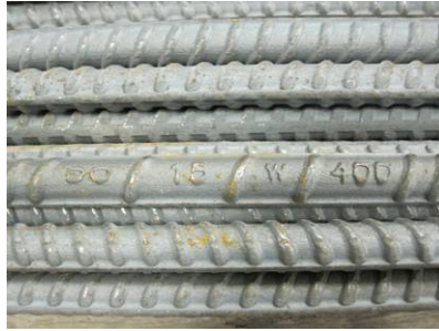
Figure 4.1 Barres d'acier 400 W – 15M
