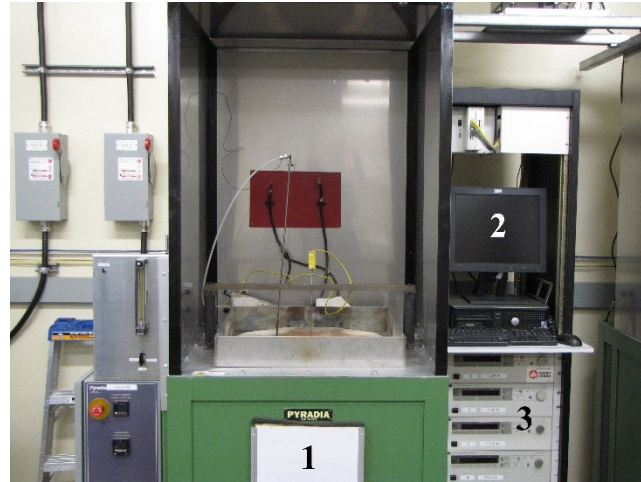
Figure 4.1 Electrolysis experimental setup with (1) oven and fume hood, (2) data acquisition and (3) power supply
