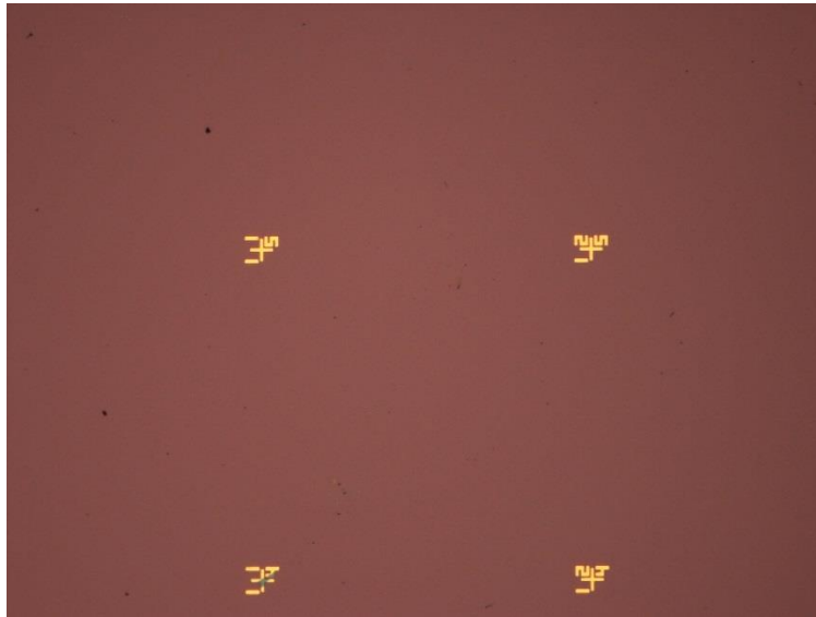
Figure 3.2. The image of Reference number patterns, transformed onto SiO 2 substrate to identify the location of nanowire while performing e-beam lithography.
