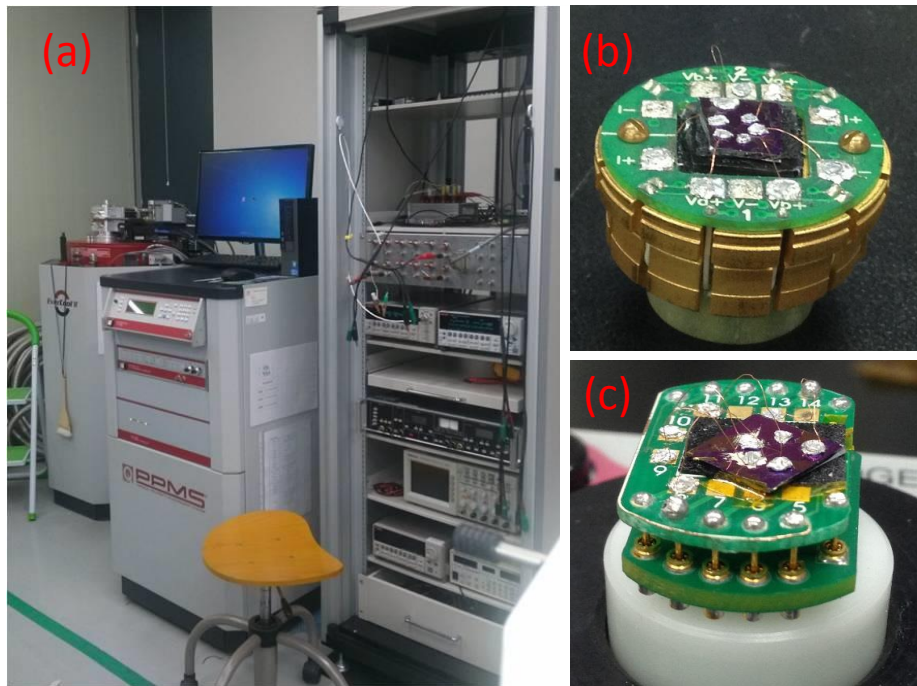
Figure 3.10. Electrical measurement setup. (a) Physical property measurement system and electric measurement setup, where the measurement was taken by using Keithley electric instrument. (b) Standard sample puck and (c) rotator puck (for angle dependent measurements) for various magnetic field ( -9 T to +9 T) and temperature dependent measurements.
