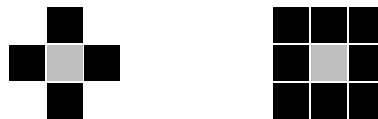
Figure 2.2: Von Neumann's neighbourhood cells (left) and Moore's neighbourhood cells (right) to the central cell (grey colour)
