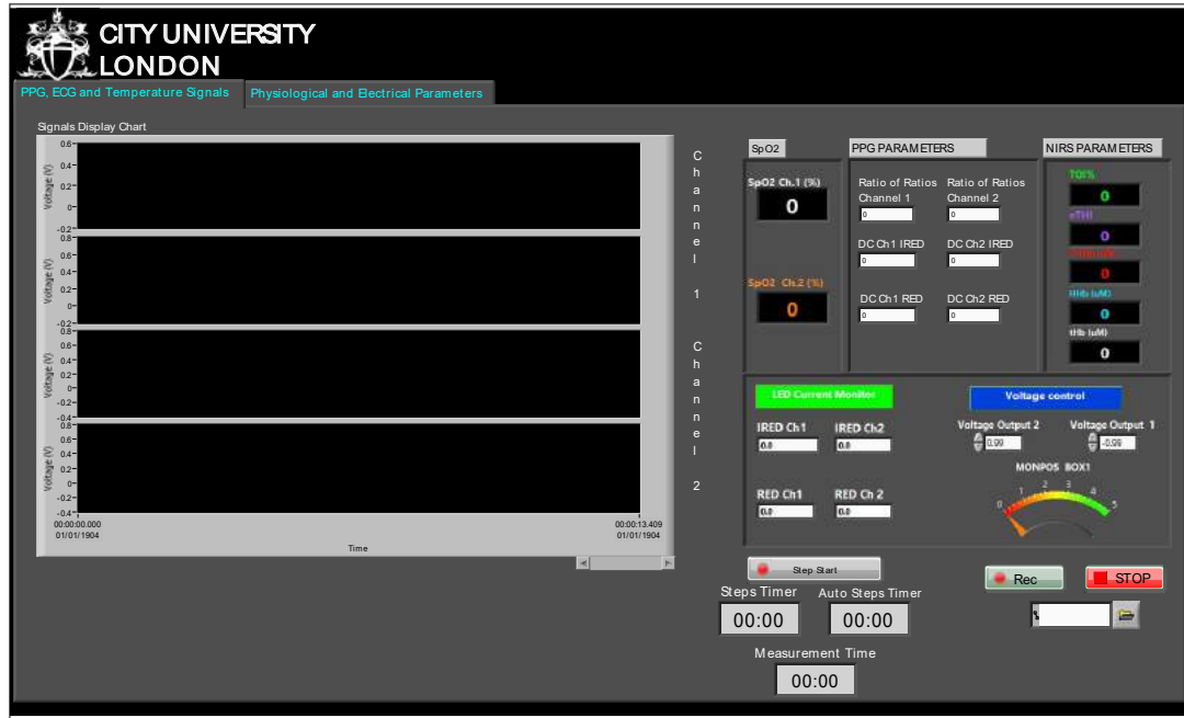
Figure 8.2: Front Panel (or user graphical interface) of the Virtual Instrument (VI) developed for acquisition of PPG and NIRS signals. The left side of the panel is dedicated to the display of the acquired signals, while indicators and controls are placed on the right side.
