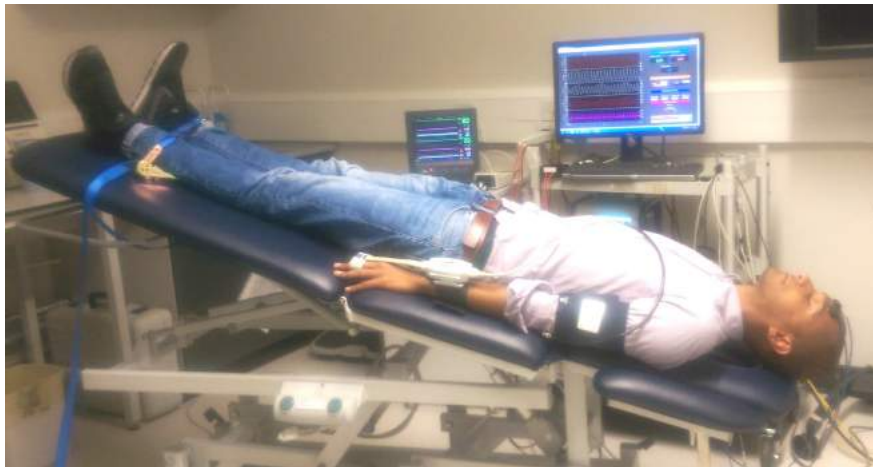
Figure 10.1: Positioning of the PPG and NIRS sensors on the forehead (a) and investigation set-up (b). The first PPG sensor (PPG-1) was placed on top of the supratrochlear vein, while the second PPG sensor (PPG-2) was placed over the eyebrow, distant from any large vasculature. The NIRS sensor was placed lateral and opposite to the PPG-2 sensor, distant from any large vasculature. The bed was tilted -30 deg as showed in (b) for five minutes.
