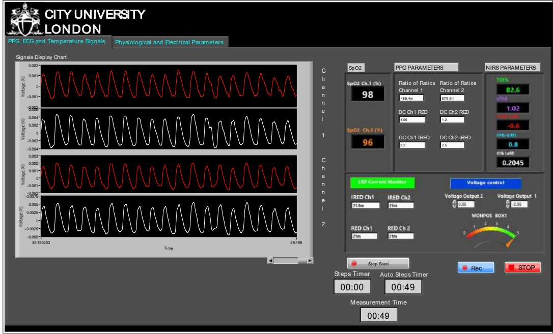
Figure 8.9: Front panel of the running VI. The PPG signals are displayed on a chart, while NIRS and other parameter are displayed as numerical or visual indicators.
