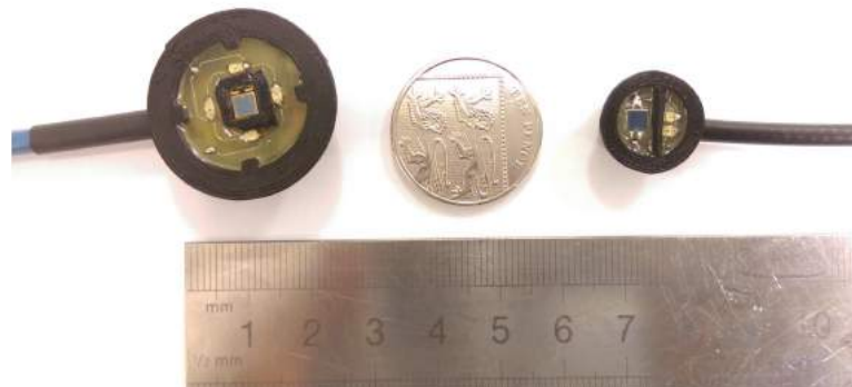
Figure 6.14: Picture of the final manufactured RPS1 (left) and RPS3 (right) PPG sensors.
