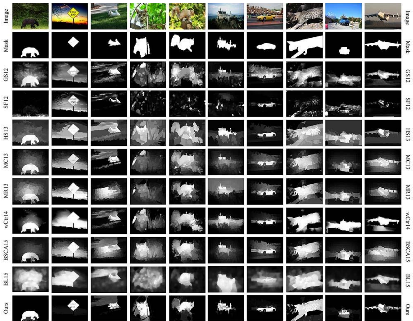
Fig. 6. Comparison of saliency maps with eight state-of-the-art methods. From top to bottom: Input images, ground-truth, saliency maps generated by GS12 [31], SF12 [30], HS13 [35], MC13 [14], MR13 [15], wCtr14 [18], BSCA15 [21], BL15 [36] and our method. Note that the proposed method generates more reasonable saliency maps compared with the state-of-the-art.
