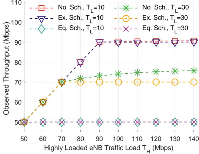
Figure 4.4: Observed Average Throughput of Highly Loaded eNBs.
