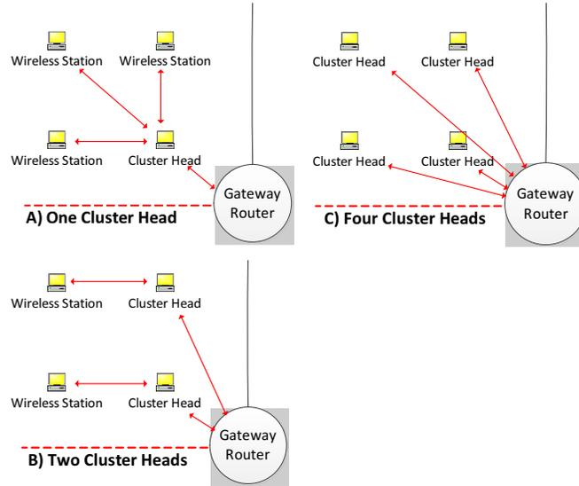
Figure 2.2: Illustration of Clustered Routing With Different Numbers of Cluster Heads in a Zone: Wireless Nodes Direct All Communication With Nodes Outside the Zone Through a Cluster Head. The Cluster Communicates With the Gateway Router, Which Is Connected to an ONU. The Configuration With 4 Heads Corresponds Effectively to an Unclustered Benchmark As All Nodes Communicate Directly (Without Going Through a Cluster Head) With the Gateway Router.
