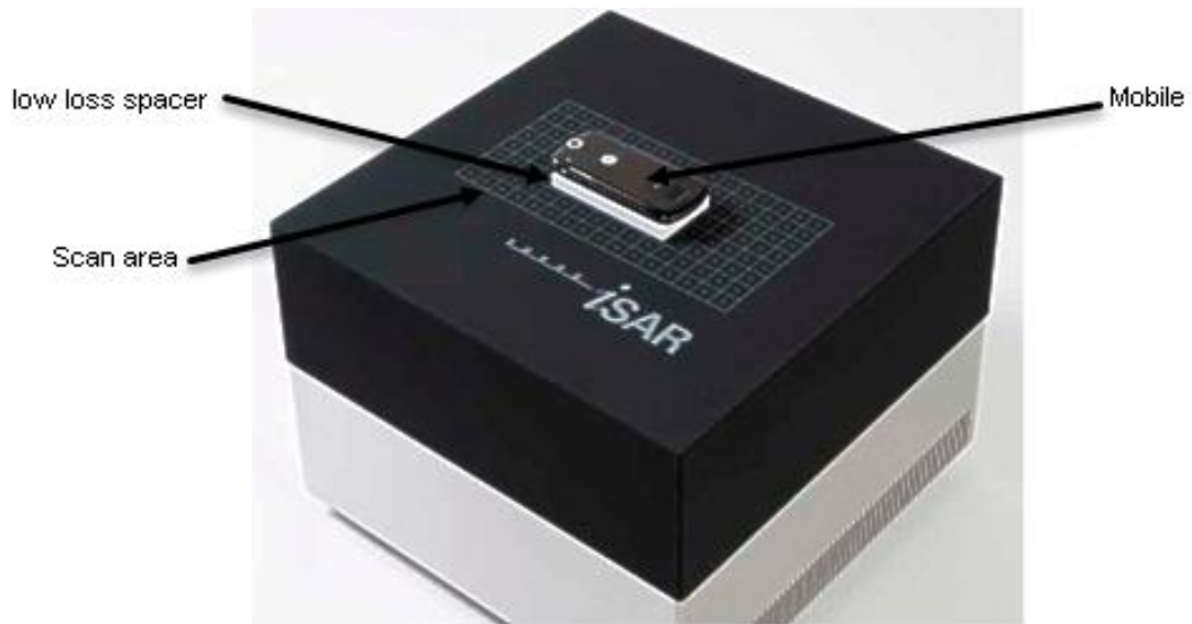
Figure 2-10: Mobile phone 2-D SAR measurement system which consists of an array of E-field probes located 4mm below the surface. After [14]
