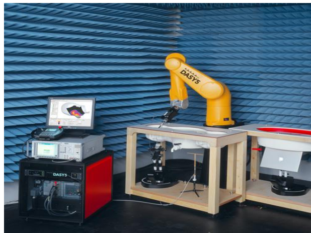
Figure 2-7: Mobile phone SAR measurement system which consists of an E-field probe positioned by a robot in a head phantom exposed to a mobile phone at the right ear. From [10]
