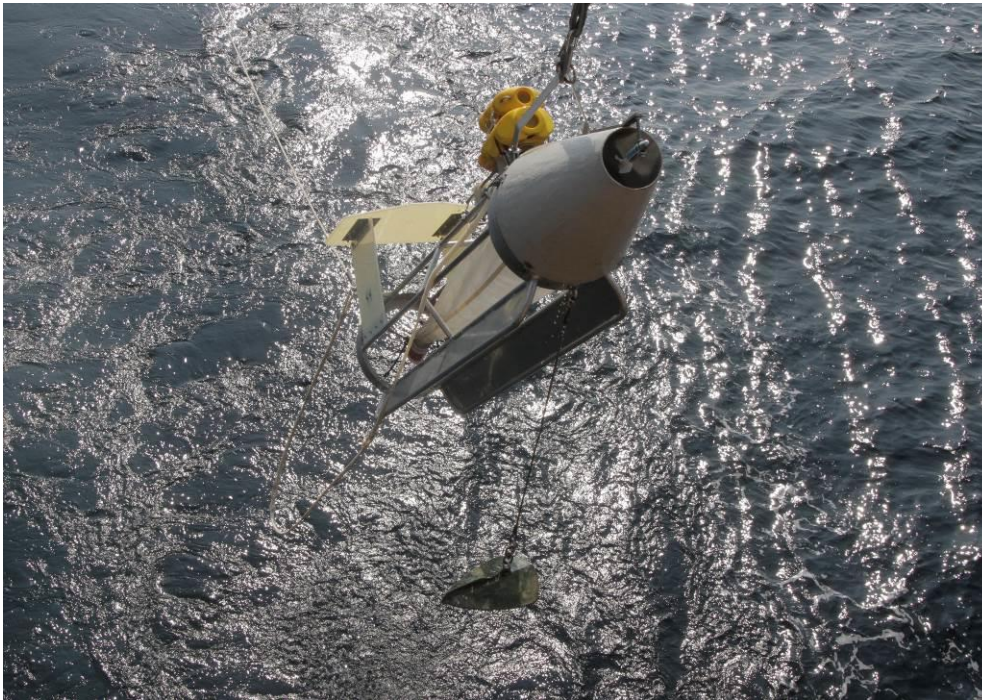
Figure 3.1 Gulf VII high speed plankton sampler with Marport depth sensors and General Oceanics flowmeter in the nosecone.
