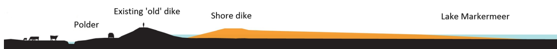
Fig. 2 Cross-section of a ‘Basic Flood Protection’ shore dike (Van der Linde et al. 2012)
