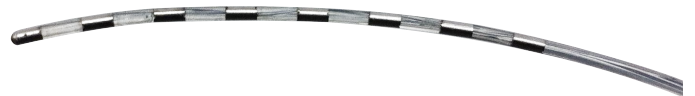
Fig. 1. Distal end of a 62 cm SCS “Octrode lead”. Eight platinum electrodes, each 3 mm long and 1.3 mm in diameter, are separated by 4 mm insulating spacers. Electrode numbering starts from ‘1’ (left-most electrode) to ‘8’ (right-most electrode).
