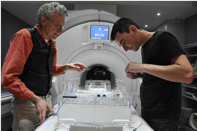
Fig. 3. Operators preparing a wire sample for testing within a gelled saline phantom in a 3T MRI machine.
