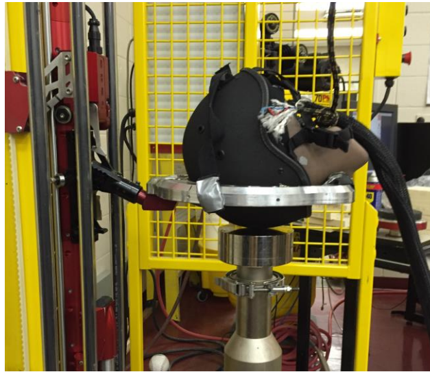
Figure 1: Monorail drop system used for unrestrained drops
