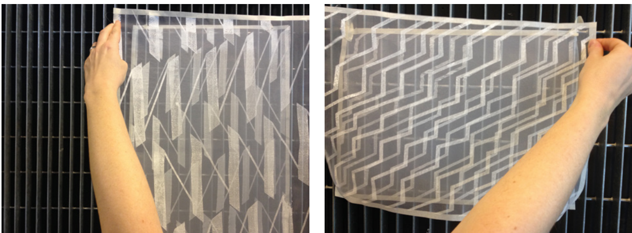
Fig. 3.25 Screen-printed textile prototypes for AJ6 . These confuse depth perception and create dynamic effects as one walks past.
