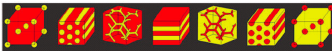
Figure 3. Morphologies of diblock copolymers. From left to right structures include spheres, hexagonal cylinders, cubic bicontinuous gyroid and lamellar morphologies 52 .
