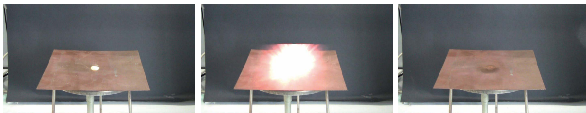
Figure 2.11: Hot-plate test of potassium 5-azido-3-nitro-1,2,4-triazolate ( 6 , 200 mg) on a copper plate, heated with a Bunsen burner. A deep dent is visible in the former place of the substance.
