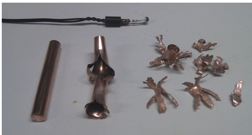
Figure 8.5: Copper tube test of 77 . Top: type A igniter; left: empty copper tube; middle: damaged copper tube after deflagration of pure 77 (100 mg); right: remnants after detonation (300 mg RDX, 50 mg 77 ).
