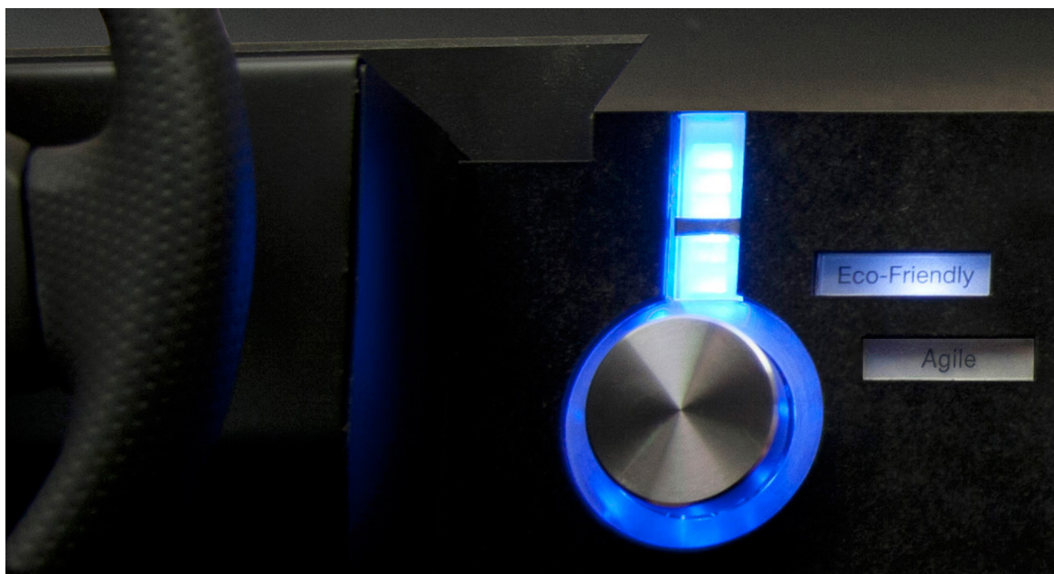
Figure 5.7: The second experience prototype Implementing Heartbeat as a start-stop-button and control element to change the driving mode between Eco-Friendly and Agile. The energy scale is located above.
