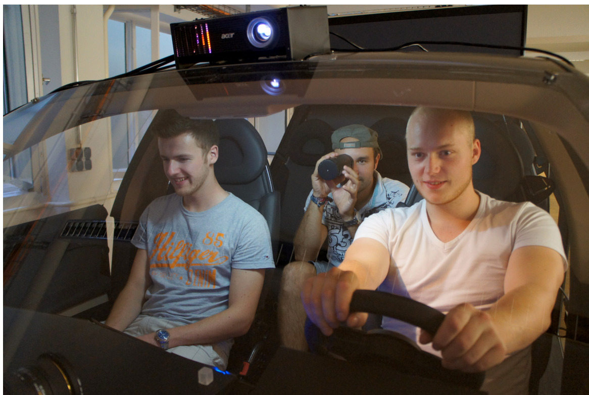
Figure 6.11: Second Periscope experience prototype used during the second user study. The passenger in the back explores points of interest and communicates his discoveries to the other passengers.
