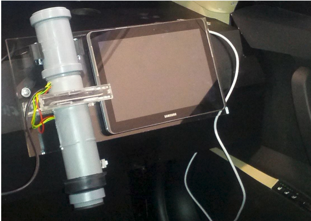
Figure 6.5: The first Periscope experience prototype and a display providing additional information about discovered points of interested are placed in the dashboard in front of the co-driver.
