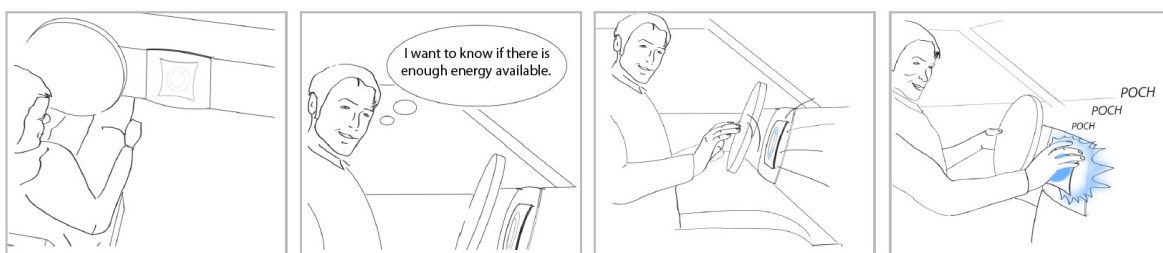
Figure 5.3: Storyboard inspired by the first Heartbeat prototype showing how a driver checks the state of the electric drive by placing his hand on the prototype to feel tactile feedback. Drawn by Marc Landau.
