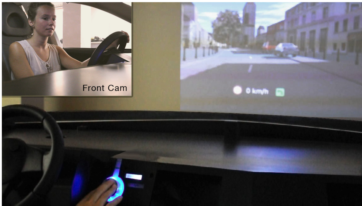
Figure 5.8: Evaluation of the second Heartbeat experience prototype. A driving simulation is projected onto the wall. The participant touches Heartbeat to feel the tactile feedback.
