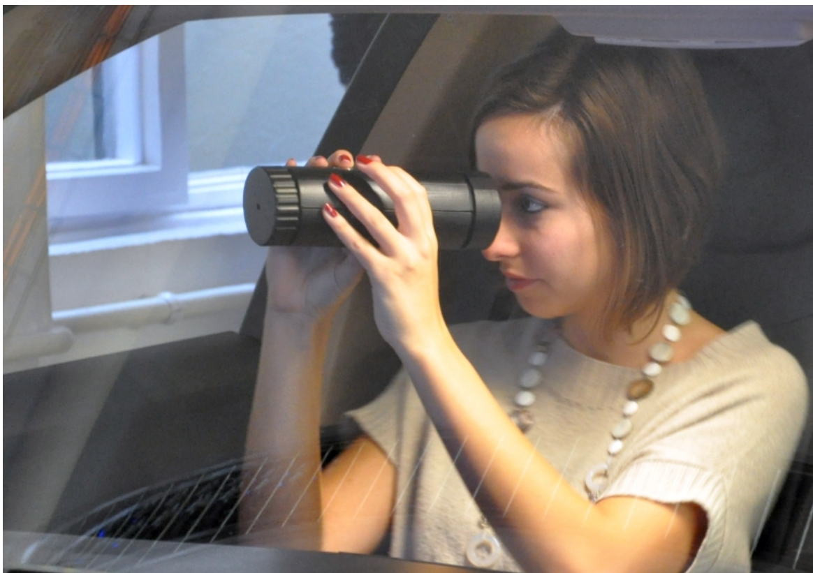
Figure 6.10: The second Periscope experience prototype. The co-driver clicks a button to freeze the image showing a point of interest she just discovered before passing on the prototype to a passenger in the back.
