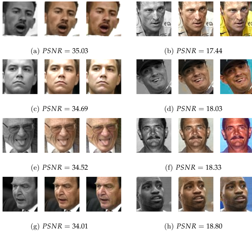
Figure 33: Images with the best PSNR on the left and with the worst PSNR on the right. Each block, columns from left to right: Grayscale image, Colorized image, Ground truth
