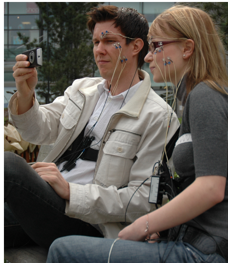
Figure 3.5: Facial EMG measurement over the brow, periocular, and cheek muscle areas via a mobile physiological data collection system in a real-world context.
