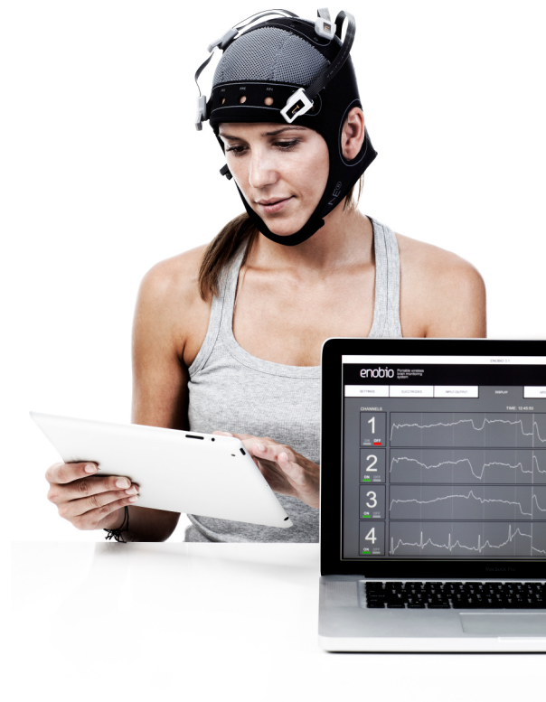
Figure 1.1: An example of an ambulatory psychophysiological set-up with an EEG amplifier plus mobile and fixed devices. Image reproduced with permission from Neuroelectrics SLU (Barcelona, Spain).
