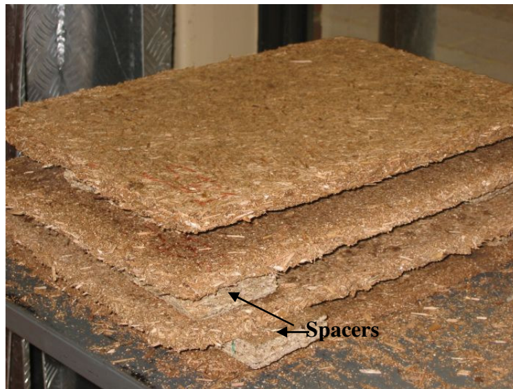
Figure 4.17: Final particleboards (before cutting and sampling)
