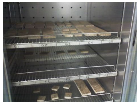
Figure 4.19b: Samples in the humidity cabinet
