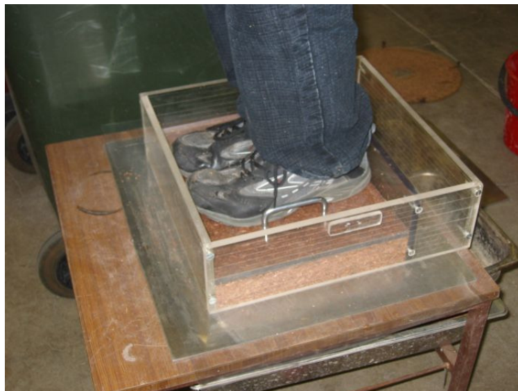
Figure 4.13: Manual pressing of the mat
