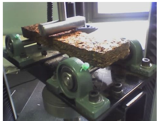
Figure 4.25b: Wet bending test
