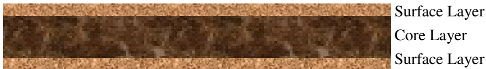
Figure 2.4: Typical cross section of a three-layer particleboard
