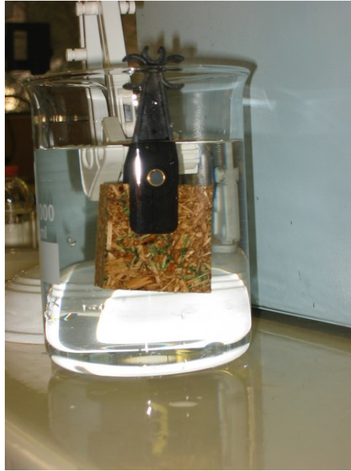
Figure 4.24: Thickness swelling test
