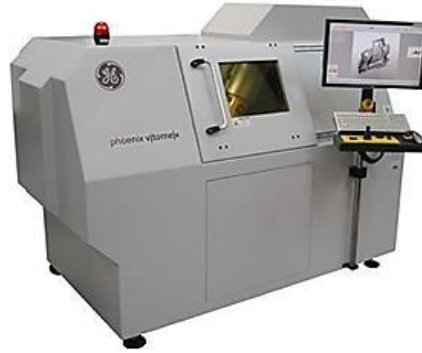
Figure 5.3. GE Phoenix v/tome/x X-ray CT machine.
