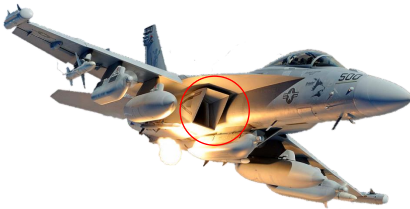
Figure 2.2. Super Hornet F/A-18E/F fighter: Carbon fibre composite z-pins used in the air inlet ducts, which is circled.
