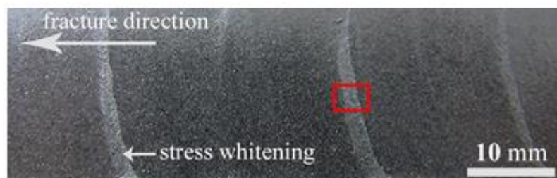
Figure 3-7 : Photograph of the crack fronts on the fracture surface of an epoxy nanocomposite with 1.0 wt% aligned CNFs.
