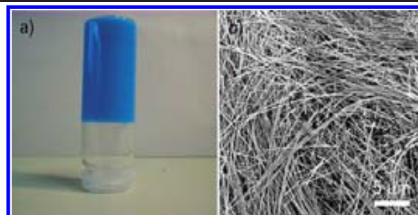
Figure 3. (a) Photograph and (b) FESEM image of the Cu-Asp-based gel.
