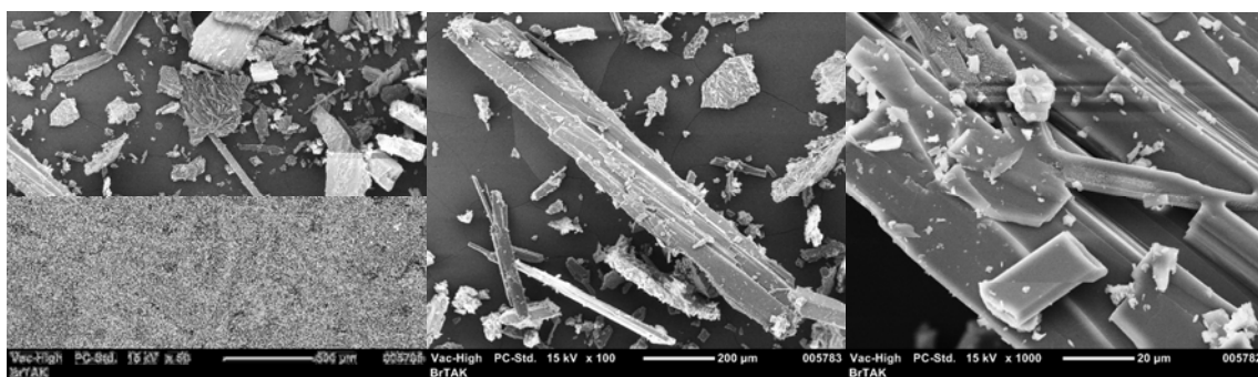
Figure III - 71. SEM pictures of the initial powder of BrTAK.
