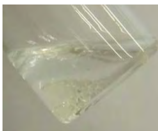
Figure III - 12. Demixion of tBuTAK in a 65/35 methanol/water mixture.
