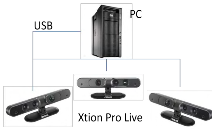
Figure 5-15 : Architecture PC Architecture PC multi Capteurs (PC HP 46 -XtionProLive 47 ).
