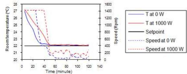
Figure 13 Motor speed and temperature responses at Tsetpoint = 22°C for PI control
