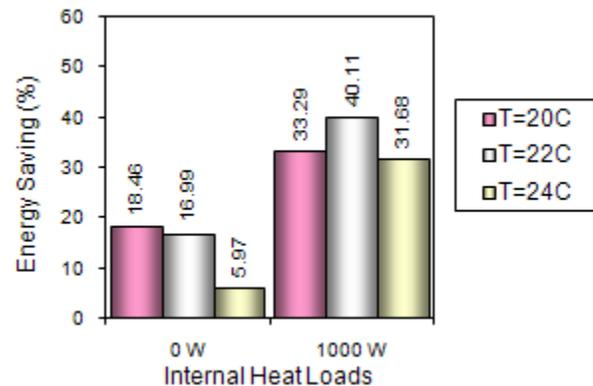
Figure 17 Energy saving distribution: on/off – PI controller
