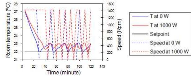
**Figure 9** Motor speed and temperature responses Tsetpoint = 22°C
