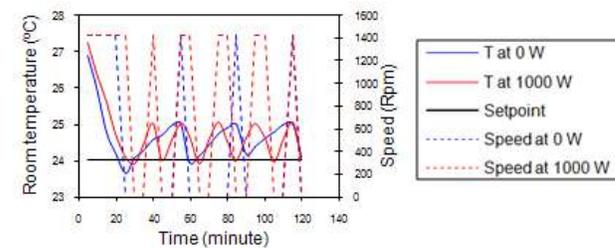
**Figure 10** Motor speed and temperature responses Tsetpoint = 24°C
