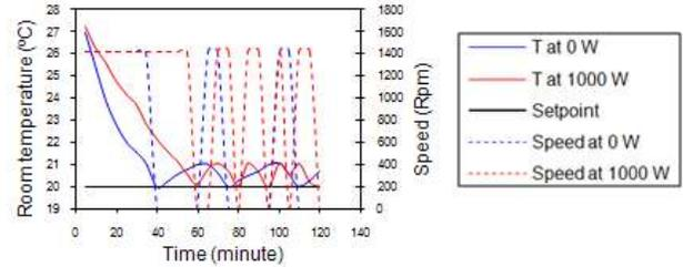
**Figure 8** Motor speed and temperature responses Tsetpoint = 20°C
