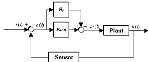
Figure 1 Block diagram of a PI control system
