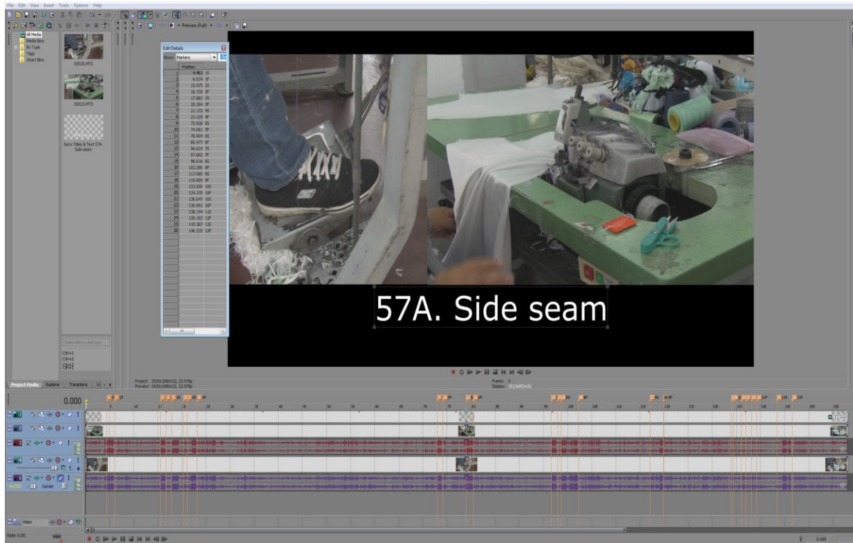
Figure 3.2 Determining sewing machine utilizing percent through using markers
